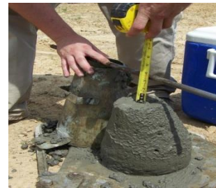
SLUMP CONE TEST
