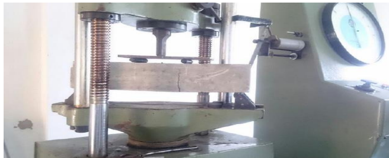
Fig. 2: Specimen loading for flexural strength test
