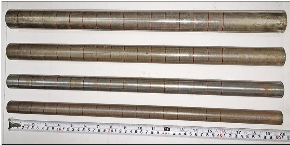
Plate 1: Pipe piles models.
