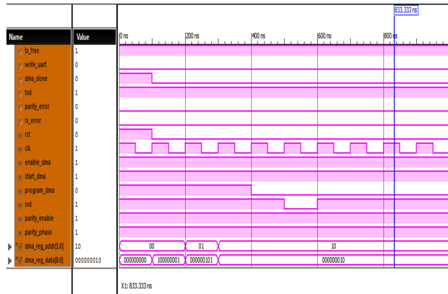
Fig 6: Simulation Result of DMA with AHB and UART
