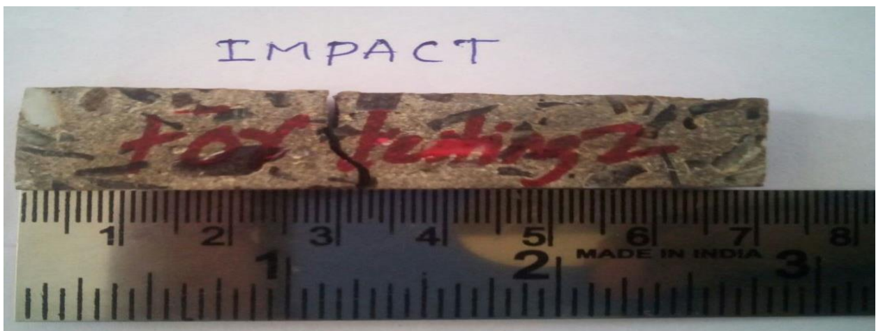
Fig. 4 Cracked DRFP composite specimen under impact test.
