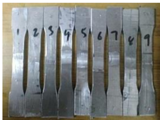
Fig. 3.7 Tensile test specimen before failure
