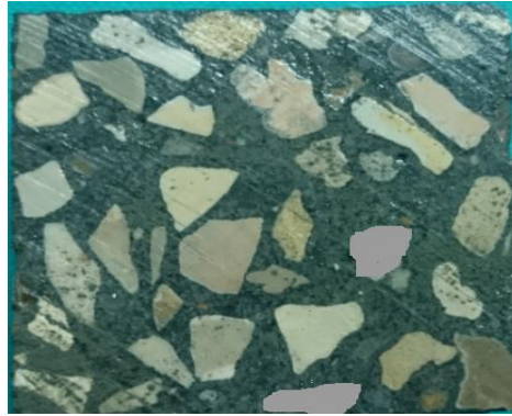
Figure 1. Distribution of coarse aggregates on cross section
