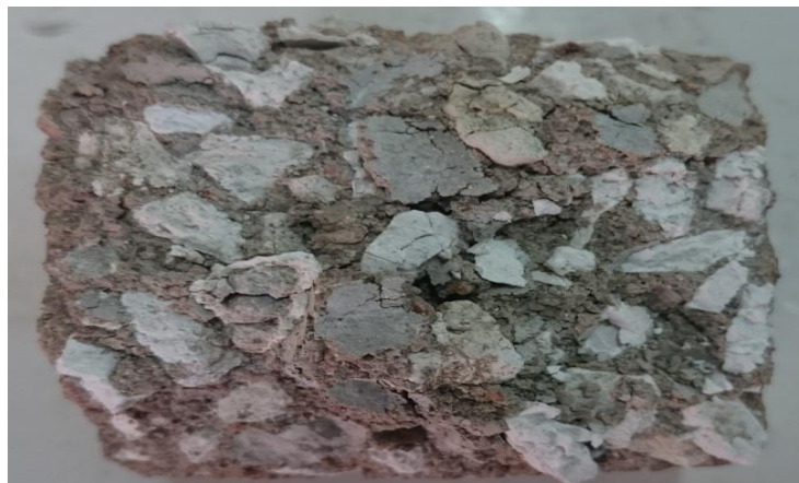
Figure 4. The decomposition of the aggregate above 800 °C
