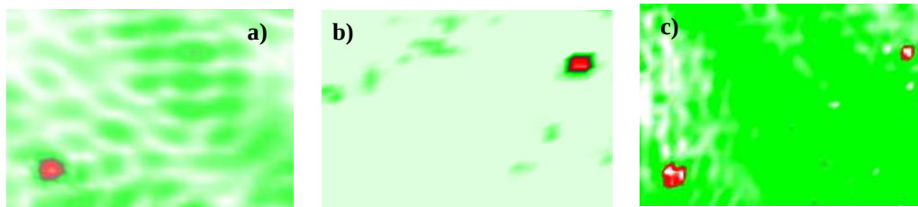
Fig. 13. Frequency-selective defect imaging of delaminations in CFRP plate in a linear LDR mode: excitation frequency 71250 Hz (a); 91130 Hz (b); frequency sweep 45-100 Hz (c).
